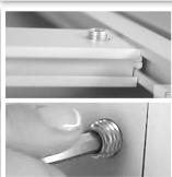
Now put the stabilizer in the frame while the lock is inserted in the inner slot of the profile. Then tighten the screws of the lock.
