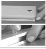
This could also be done after the frame mounting, but it is easier if only 3 profiles are connected. Prepare the stabilizers by inserting the locks in the stabilizer, so the holes of the lock and the stabilizer are above each other.
