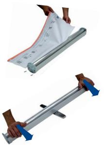
**3** - Unfold the stabilizing foot. Place your palms at the outer ends of the roll. Tension the spring mechanism 39 turns by sliding your palms forward.
