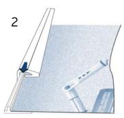
Slide the top profile onto the graphic panel.
