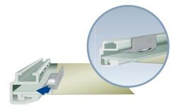
Turn the image around and push the clips into the places marked with a black line at the top profile.
