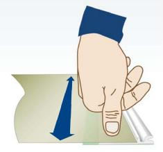
Remove the remaining part of the protective liner and press the image firmly onto the panelstrip.
