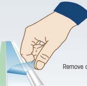
Remove a small part of the protective liner on the fronttape.
