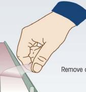
Remove a small part of the protective liner on the fronttape.
