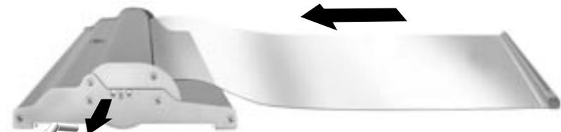
Slow down the image with one hand when pulling out the locking key.
