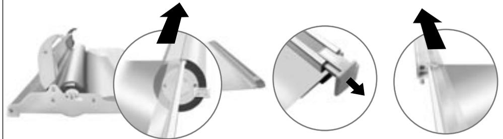
Take out the roll and remove the existing image by pulling off the roll and the top profile.
