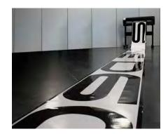
Summa's automated contour alignment system OPOS stands for Optical Positioning System. The OPOS sensor registers printed squares around the graphic. This allows OPOS to determine the exact position of the printed graphic and enables you to die-cut valuable printed and laminated vinyl graphics with complete confidence and ease.
