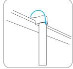
9. Locate the back channel of the snap rail onto the plastic adaptor at the top of the pole. Repeat steps in reverse to disassemble.
