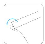
3. Push the snap rail closed ensuring the media is secure.
