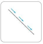
8. Remove the telescopic pole and fully extend. Push each section into the next to lock into place.
