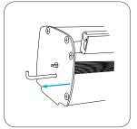
5. Hold the snap rail and the cassette securly and remove the pin from the side of the cassette to engage the mechanism.
