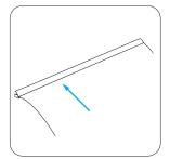
2. Slide media into the bottom end of the snap rail.
