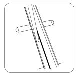
10. Ensure the pole is located onto the plastic lug securely. The lug sits inside the channel below the pole insert hole.
