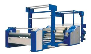
The production lines can be equipped with driven and tension(less) controlled winding and unwinding positions, web guiding and edge cutting equipment, accumulators or scray's for uninterrupted production. With the proper options, all kind of materials can be processed: Woven, non woven, knitted or stretch materials, thin or thick.
